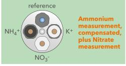
(Possible) configuration of VARiON®Plus 700 IQ for ammonium measurement dynamically compensated plus nitrate measurement (manuel compensation possible)
